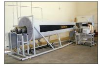
Anemometers are wind-tunnel tested in our California factory.
