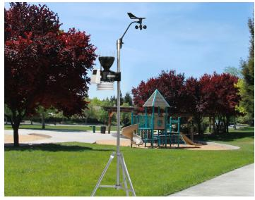
Vantage Pro2 on Mounting Tripod
