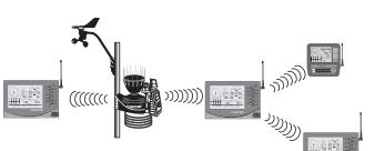
Use your console as a repeater to transmit data from one console/receiver to another.
